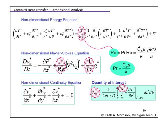
According to our **dimensional analysis** calculations, the dimensionless heat transfer coefficient should be found to be a function of <u>four</u> dimensionless groups:
