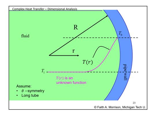
At the boundary, (Newton's Law of Cooling is the boundary condition)
