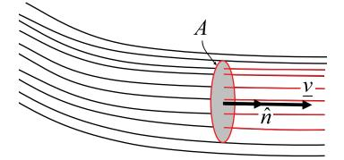
Figure 3.24: For this example we consider the flow through a surface A. The velocity of the fluid is perpendicular to the surface A.
