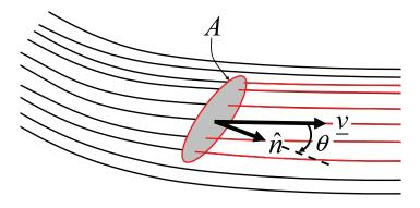
Figure 3.26: For this example we consider the flow through a surface A. The velocity of the fluid is not perpendicular to the surface A; instead, the velocity makes an angle  $\theta$  with the surface unit normal  $\hat{n}$ .
