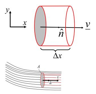
Figure 3.25: During the time interval  $\Delta t$ , a volume of fluid of height  $\Delta x$  and of cross-sectional area A passes through the area A.
