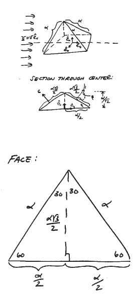
Figure 3.28: The control volume is a square pyramid, which has five sides, four of which are equilateral triangles.
