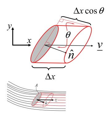
Figure 3.27: During the time interval  $\Delta t$ , a volume of fluid of height  $\Delta x \cos \theta$  and of cross-sectional area A passes through the area A.
