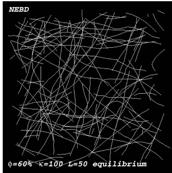
Fig. 26. Equilibrium high density semiflexible FENE-B chains (48) for system parameters given in the figure.
