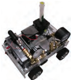
Fuel cell-powered Chem-E-Car
