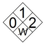
The area with a "0" in the diamond denotes health hazard, the area with the "1" denotes fire hazard and the area with a "2" denotes reactivity hazards. The box at the bottom is used to denote special hazards, e.g. incompatible with water.
