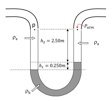
Note: the inner diameter of the manometer tube is 11.2 *mm*.
