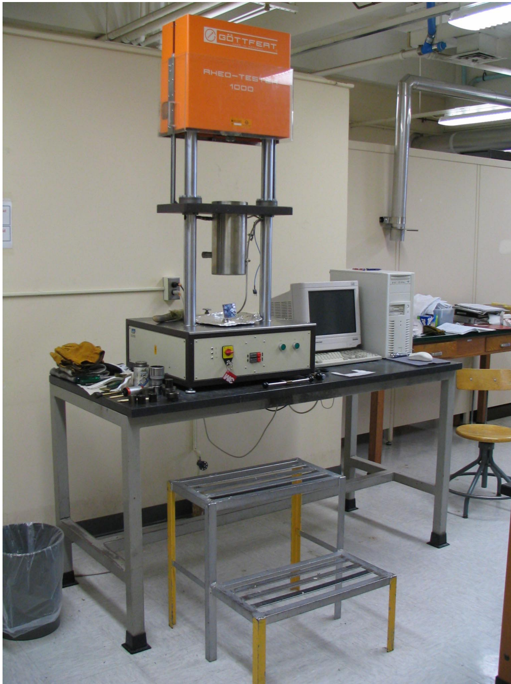
Figure 1: The Goettfert Rheotester 1000 is a bench-scale capillary rheometer. The upper orange chamber houses the hydraulic drive. The stainless steel cylinder in the center houses the barrel and the heating units for the barrel. Electronics are housed in the lower portion, and the instrument is computer-controlled.
