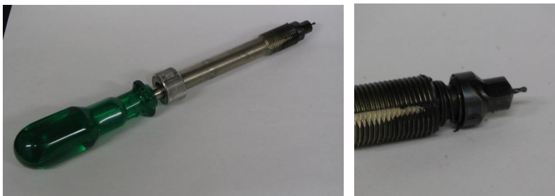
Figure 4: The cleaning tool for the pressure-transducer hole appears above. A small threaded appendage (shown at right) extends from the tip of the cleaning tool and fits into the hole that connects the plastic in the barrel to the end of the pressure transducer. Care should be taken not to break off the cleaning tip.
