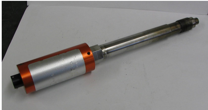
Figure 3: The 1400 bar pressure transducer is shown above. The pressure-sensing end is to the right. The orange portion houses the electronics and the connection that is made to the rheometer.
