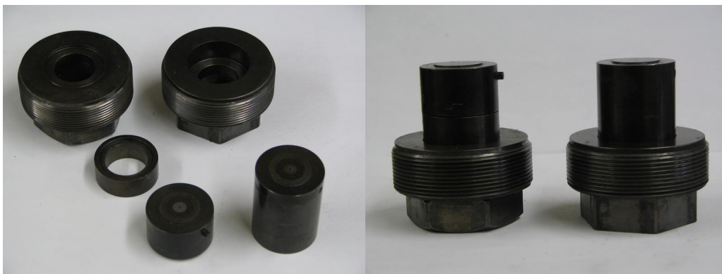
Figure 2: The 20/1 capillary and the 40/1 capillary and their capillary nuts. Note that the nut for the 40/1 capillary has a recess, while the 20/1 capillary requires a distance ring. The assembled capillaries have the same linear heights as shown at right. Note the slight elevation of the central portion, which indicates that the capillaries are in right-side up.
